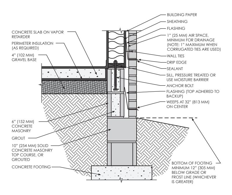
SLAB ON GRADE WITH MASONRY ABOVE GRADE CROSS SECTION
