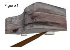
Using an appropriately rated skid steer or small excavator and the Rosetta Lifting Device, **place each block along the string line.** Be sure that the safety latch on the Lifting Device is engaged before lifting each block. (For more information about the Rosetta Lifting Device, refer to the Lifting Device Instructions.)
