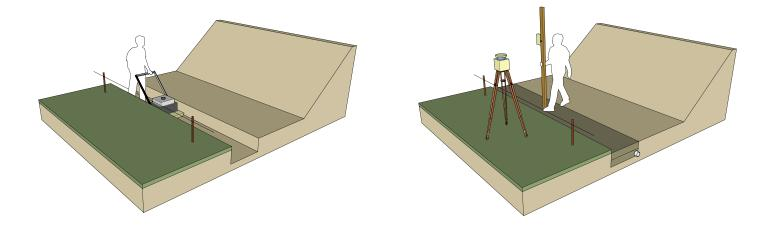
**First, excavate for the leveling pad.** The minimum leveling pad thickness is 6 inches (150 mm). Higher walls may require a thicker leveling pad based on the detailed wall design. The leveling pad should be a minimum of 36 inches (0.91 m) wide, or wider if called for in the engineered construction drawings. The subgrade material should be compacted to 95% of its standard proctor maximum dry density.
