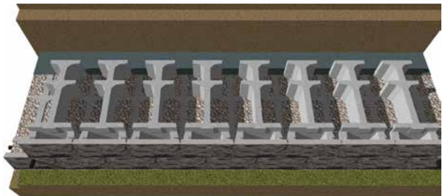
Lay the next row on a running bond pattern with the SecureLugs connected in the hollow cores of the blocks below. Complete the second row installation ensuring everything is level.
