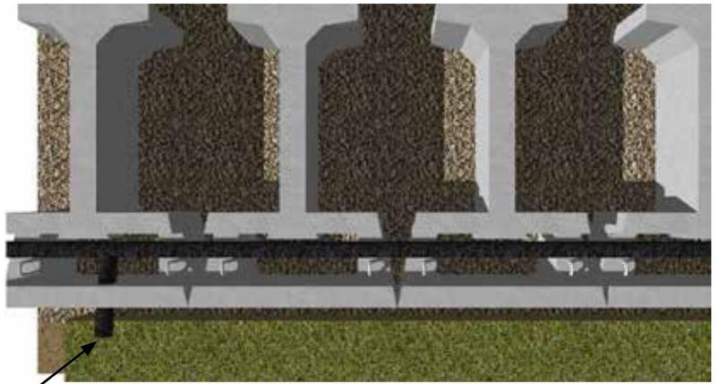
4" perforated drain pipe that daylights to front of wall a minimum of every 35 feet.
