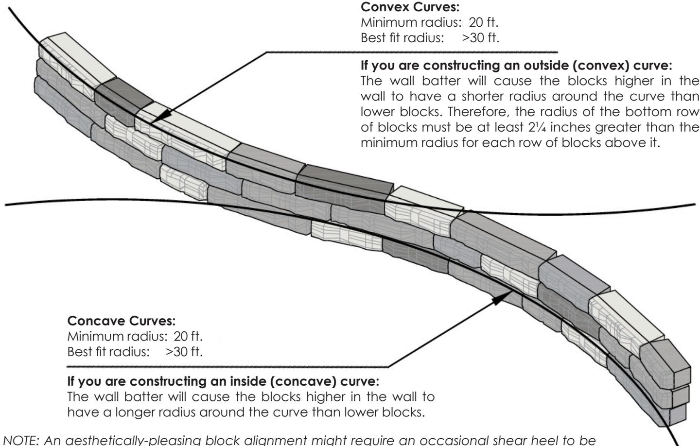
*NOTE: An aesthetically-pleasing block alignment might require an occasional shear heel to be removed to allow for a smoother curve. This is acceptable in limited amounts without significantly affecting wall structural performance.*
