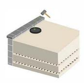
Punch the perforated lid using a mallet or hammer to expose the inside of the Sleeve-It unit. Detached lids can be leh inside the unit or discarded prior to pouring of infill material.
